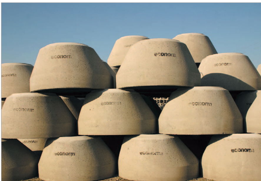
In the concrete works. econorm® units before despatch to the building site
